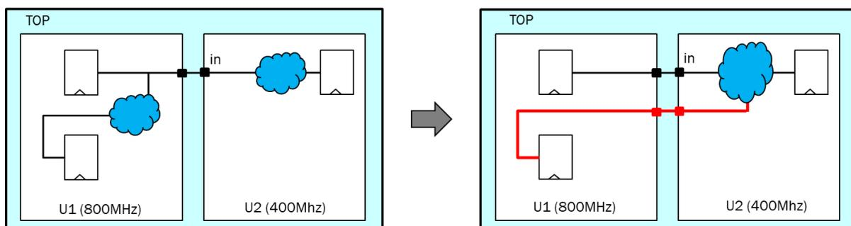
Consider the example shown in the above figure. After logic restructuring, the resulting logic is optimized by combining the logic from U1 and U2. Functionally, they are equivalent, however, from the timing point of view, the original SDC may not be valid, if applied on the resulting design. For example, if there is a timing exception placed on port "in", such as:
