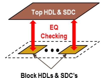
A simple case may be that the clocks are designed to be synchronous at the top level, while at the IP level, they are meant to be asynchronous. Assumed constant values set by the *set\_case\_analysis* command at the IP level may conflict with what is defined at the top level.
